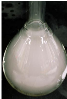
Thick mist formed sulfur trioxide + water
